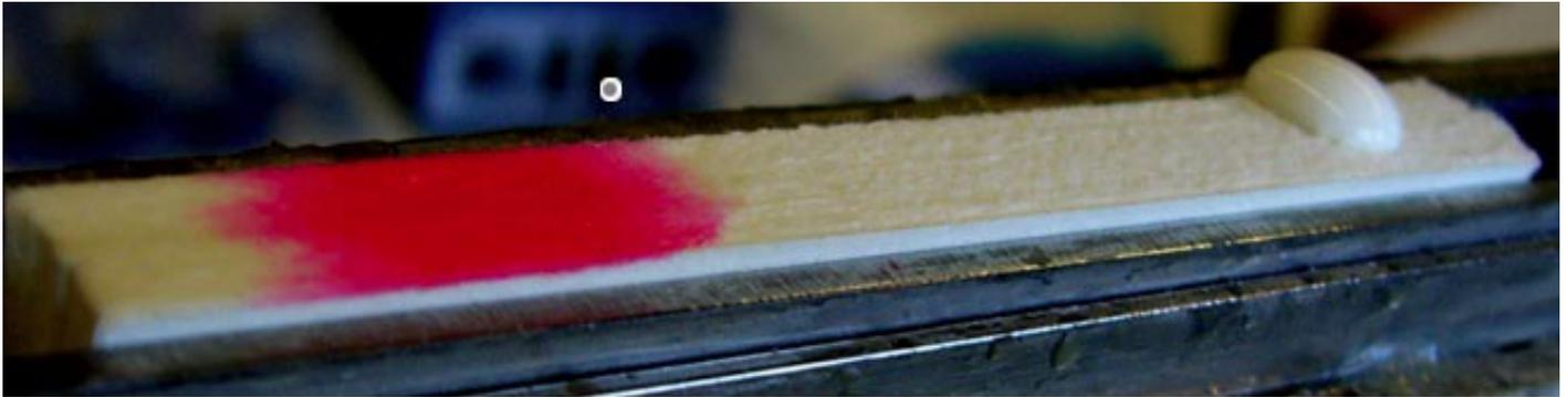
Note, the PVA glue on the right just stays on top. The left side is treated with an H\*Protein additive. The PVA adhesive, colored red is spreading, causing the unusual strong bond.
