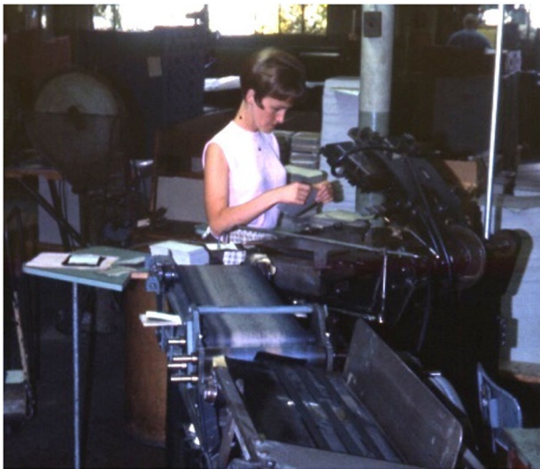
The Reece case-making machine at World Publishing. Photo courtesy of Werner Rebsamen.
