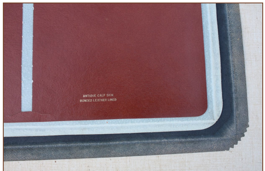
The fine and often expensive leathers are die-cut to size. The edges/turn-ins require skiving. No paper linings are used. The covers are all leather. Photo courtesy of Werner Rebsamen.
