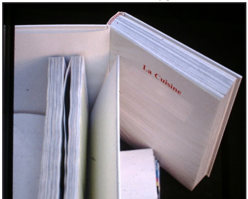
Not being familiar with the consequences of the paper grain being perpendicular to the binding edge sent these Canadian cookbooks to the grave yard. The books would not open. Note the wavy paper. Photo courtesy of Werner Rebsamen.
