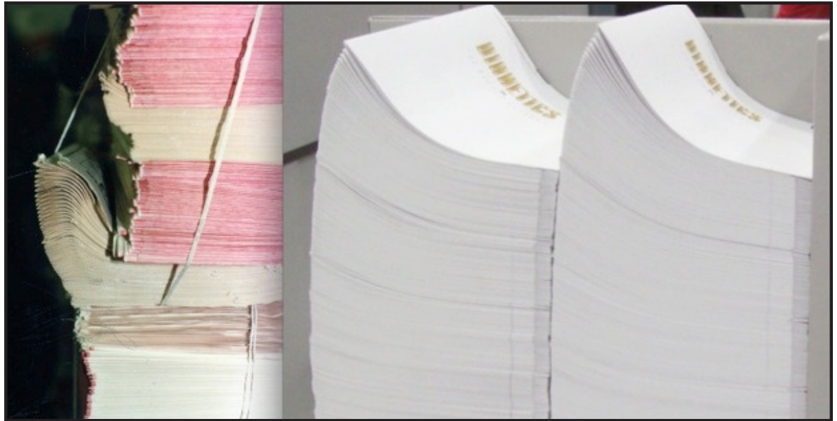
Distorted, or fluffy signatures/book blocks (right), cause costly downtime and result into poor quality bindings. On the left, signatures compliments of a commercial printer. Photos courtesy of Werner Rebsamen.
