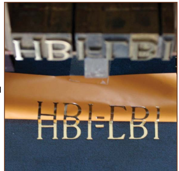
Test performed on author's hotstamping press - is the foil compatible with the substrate?
