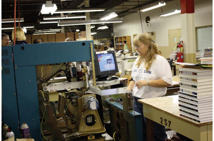
Imprinting the spines on hardcover bound books - just imagine all the possibilities, especially for photo books. For example, generic theme covers made on high speed equipment, personalized imprinting and more ( www.flesher.net ).
