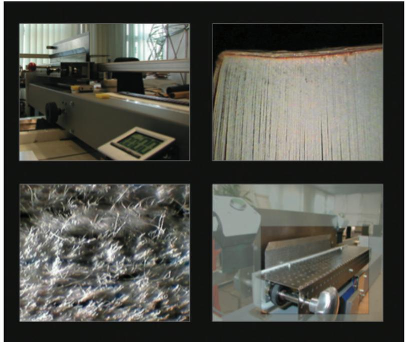
*The all-new Junior adhesive binder does feature an exclusive, patented spine preparation. Note the exposed paper fibers. A unique PVA adhesive extrusion application requires no cleaning-up. A binder ideal for high quality hard- and softcover bindings. (Ribler)*
