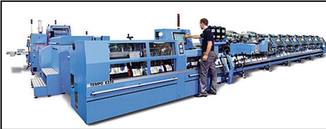
Operators like this one on a Muller Martini Tempo 220 saddle-stitch line can process up to 22,000 magazines per hour. In-line personalized ink-jet printing, inserting cards, addressing, zip-sorting etc. are all very complex, high-tech operations which require advanced skills. (Photo courtesy of Muller Martini)
