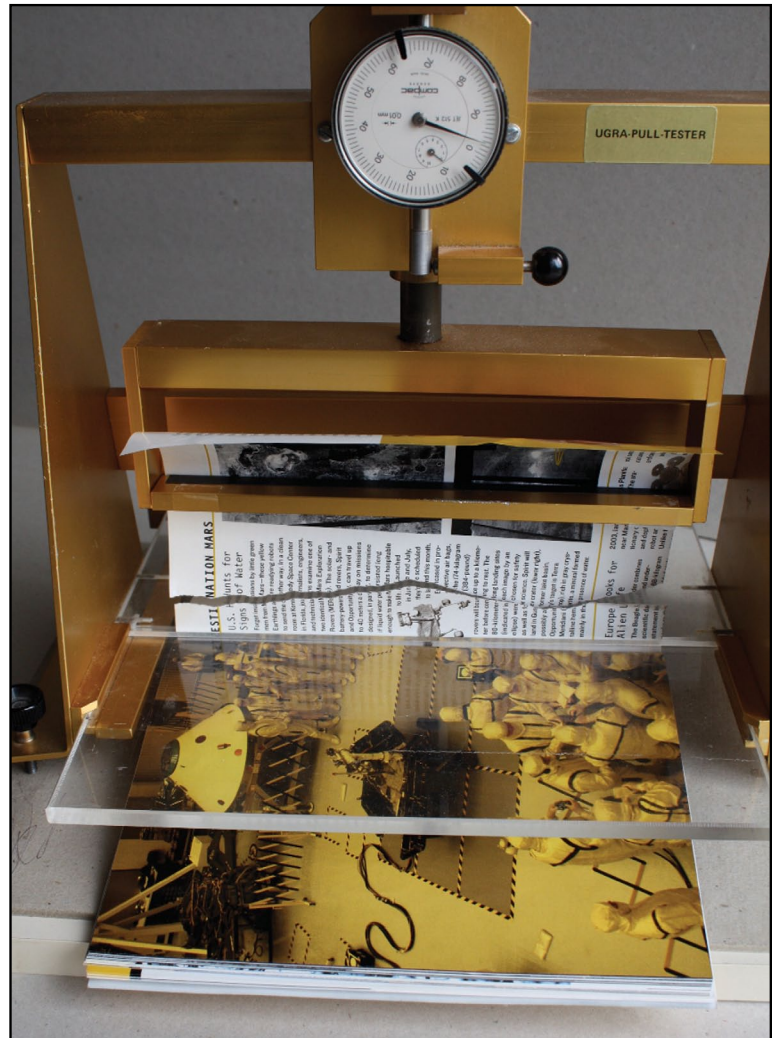
Books bound with PUR show exceptional strength. When tested for tensile page-pull, the paper is weaker than the strength of the binding.
