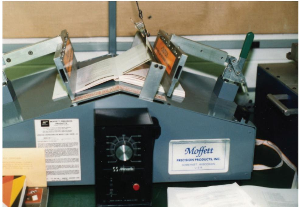
*A tensile flex test evaluates the strength of the adhesion on text blocks which must open flat.*
